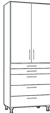
Tall 2 Door 5 Drawer Door stretches on height Drawer are all fixed height. Top two drawers are 3.585"H, bottom three are 7.366"H
