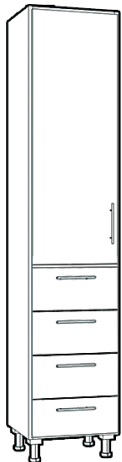
Tall 1 Door 4 Drawer Door stretches on height Drawer are all fixed height. All drawers are 7.366"H.
