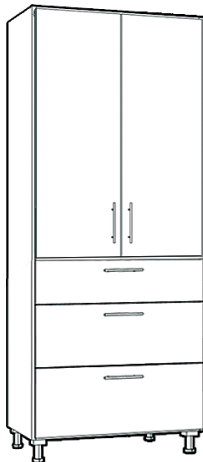
Tall 2 Door 3 Drawer Door stretches on height Drawer are all fixed height. Top drawer is 7.366"H, bottom two are 11.148"H
